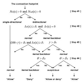
Fig. 3 The decision tree for detecting and defeating kernel backdoors.
