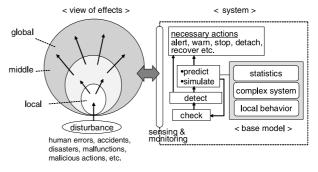
Fig. 5 Techonlogy assessment for fault tolerance.
