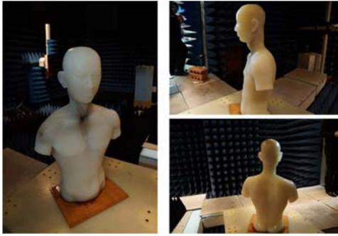
Fig. 7 Torso phantom for measurement.
