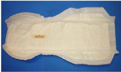
Fig. 11 Manufactured antenna on a paper diaper.
