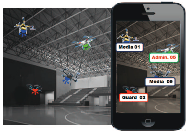
Fig.11 Drones and LED beacon.
