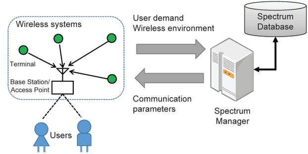
**Fig. 15** Spectrum manager with spectrum database.
