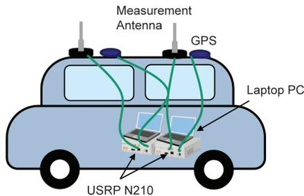
Fig. 12 Measurement devices.
