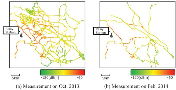
Fig. 13 Measurement-based spectrum map.
