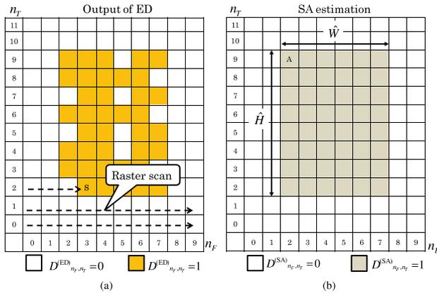
Fig. 4 Example outputs of energy detection and signal area estimation.
