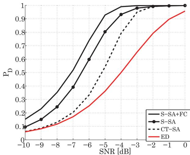
Fig. 5 Detection rate versus sound-to-noise ratio [dB].
