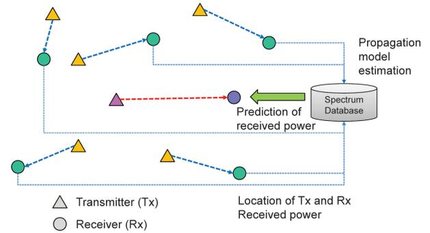
Fig. 10 Distributed measurement-based propagation modeling.
