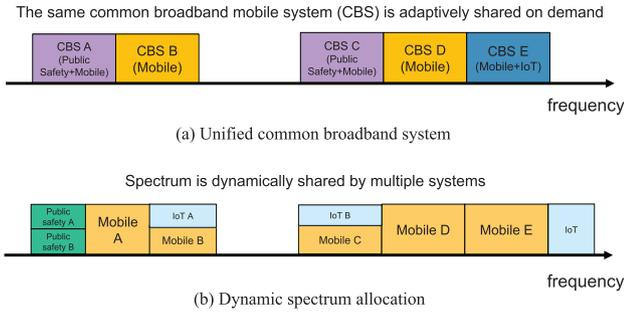
**Fig. 14** Unified system and dynamic spectrum allocation.
