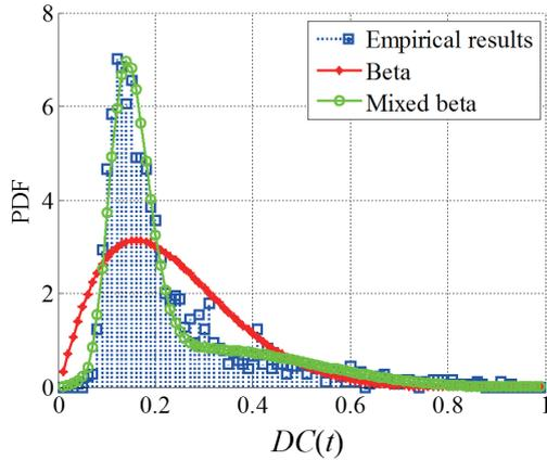
**Fig. 7** Probability density function of duty cycle ( $DC(t)$ , from  $t = 14 : 00$  to  $t = 16 : 00$ ): empirical results and stochastic models with beta distribution and mixed distribution.
