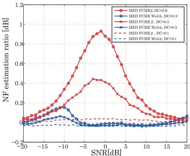
**Fig. 3** Noise floor estimation as a function of the sound-to-noise ratio [dB]. DC=0.1, 0.5 and 0.9. MED-FCME- $\beta$  and MED-FCME-Welch FFT.
