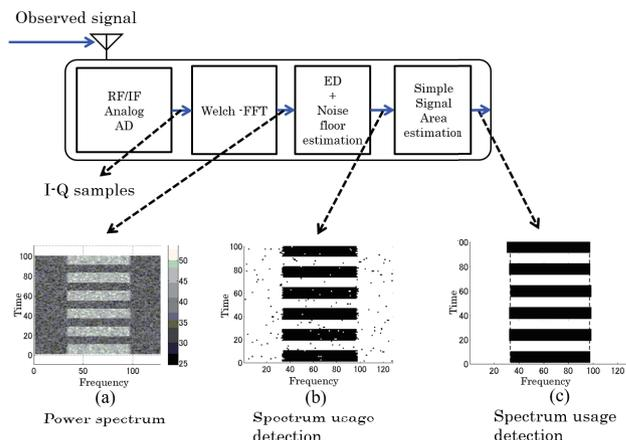
Fig. 2 Signal processing flow for spectrum measurement.
