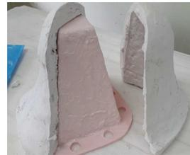
(c) Plaster molds and silicone mold.
