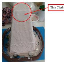
Fig. 6 Mask silicone over the pyramidal wooden mold.
