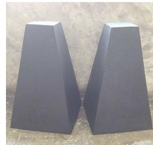
Fig. 8 New proposed absorber obtained from silicone mold.
