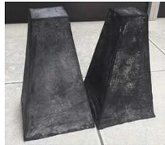
Fig. 4 Developed pyramidal EM absorber made by latex.
