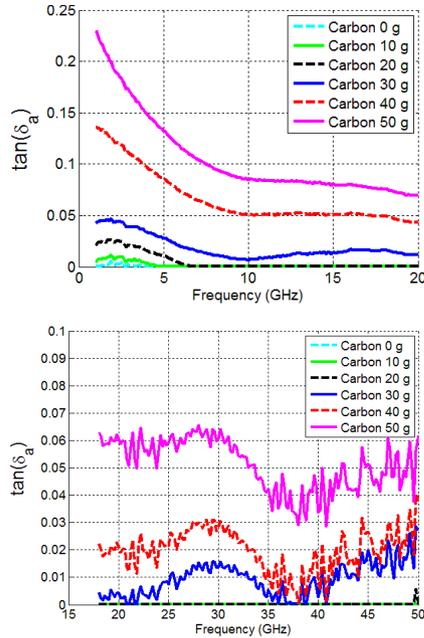
Fig. 12 Alternating electric loss tangent ( $\tan(\delta_a)$ ).
