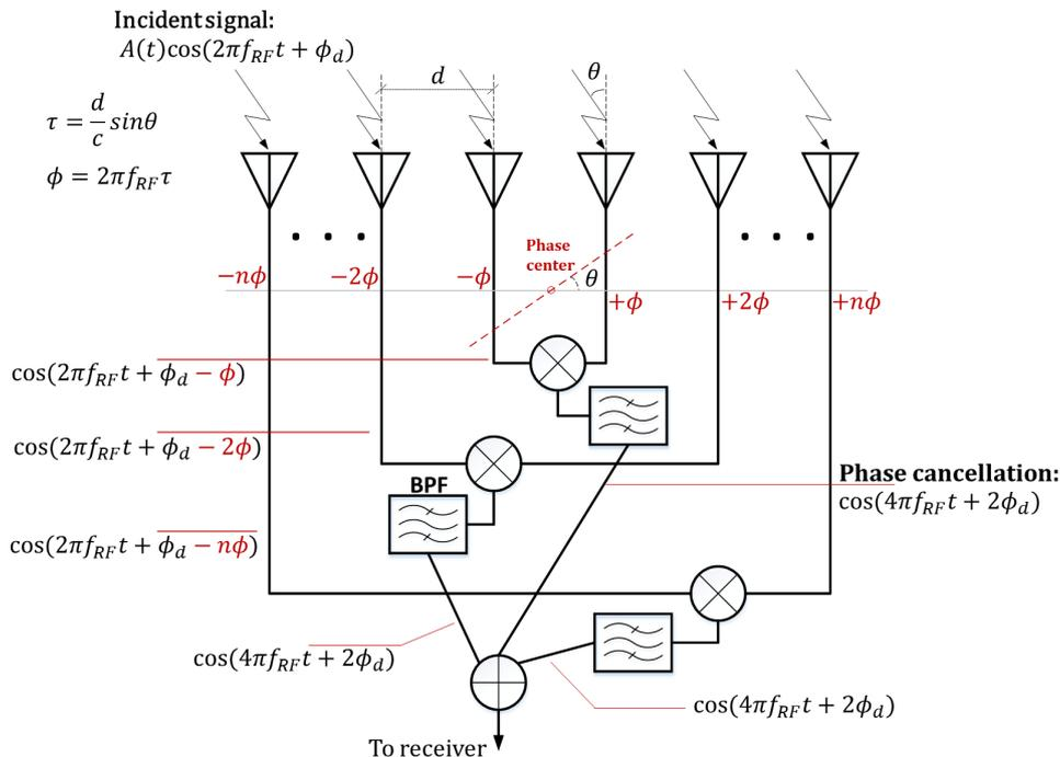
**Fig. 9** Frequency independent beamforming for the subarrays shown in Fig. 2 [14].
