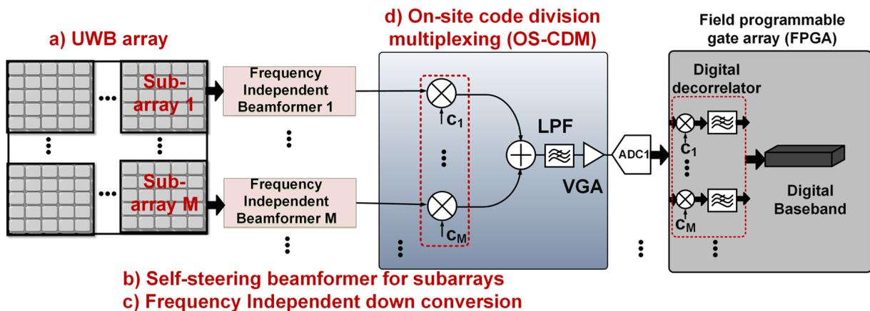
Fig. 2 Hybrid beamforming concept that combines the on-site code division multiplexing (OS-CDM) approach with subarrays for further reduction of costs in achieving frequency independent beamforming.
