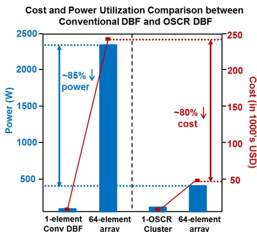
**Fig. 6** Comparison between 64-element conventional beamformer and 64-element OS-CDM in terms of cost and power. 1-OS-CDM cluster corresponds to combining 8-paths together into a single path [7].
