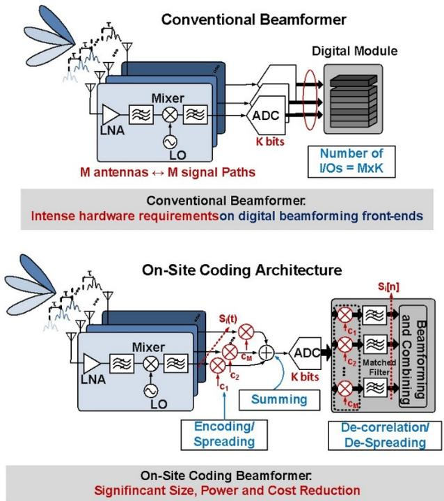
Fig. 1 Traditional beamformer using a single ADC for every antenna element (top) vs. the on-site coding scheme that uses one ADC to serve several antennas concurrently (bottom).
