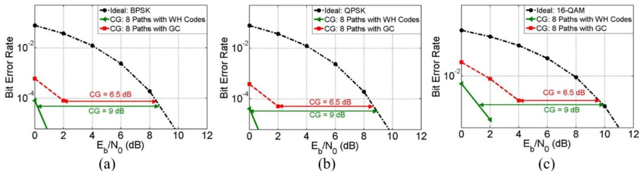
**Fig. 7** BER analysis of an eight-channel OS-CDM for various modulation schemes when Walsh-Hadamard (WH) and Gold Codes (GC). The computer BER and combined gain (CG) are compared with theoretical limits for the same modulation scheme (shown in black): (a) BPSK, (b) QPSK, and (c) 16-QAM [7].
