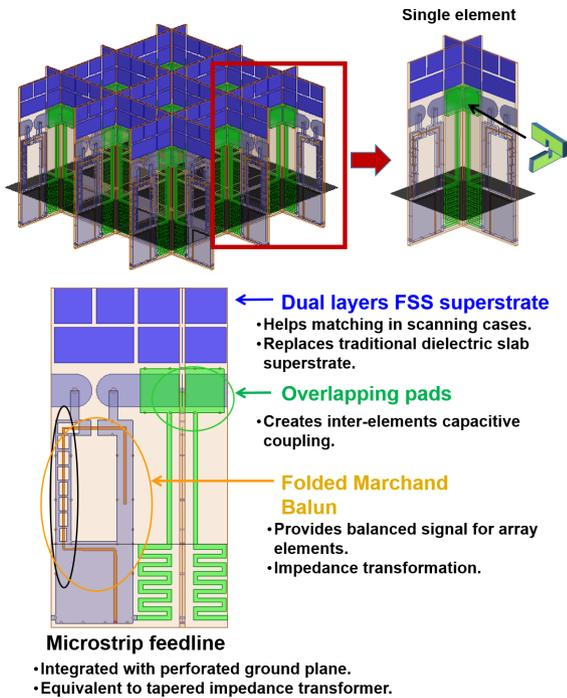
**Fig. 3** Tightly coupled dipole array (TCDA) [4], [5], [8]–[11] rendering and details of the wideband feed structure. More than 9:1 bandwidth has been achieved by these conformal arrays. Also, the arrays are scalable from low MHz up to 90 GHz using PCB fabrication processes.
