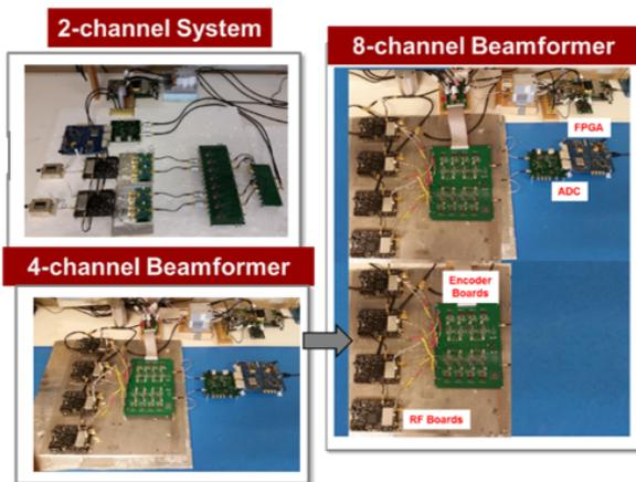
**Fig. 8** Fabricated prototypes of 2, 4, and 8-channel OS-CDM receiver using a single ADC [6], [7], [12], [13].
