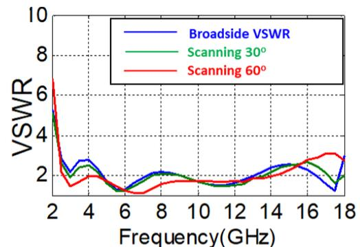
**Fig. 5** VSWR of the array in Fig. 3 for different scan angles down to 60°.
