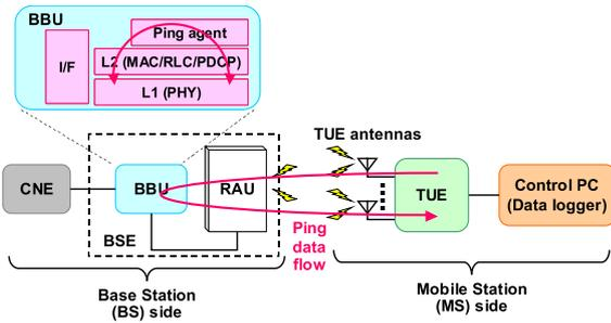
Fig. 4 Fundamental system configuration of 5G prototype for field trial.
