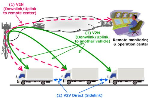
Fig. 3 Types of vehicular communication in truck platooning.
