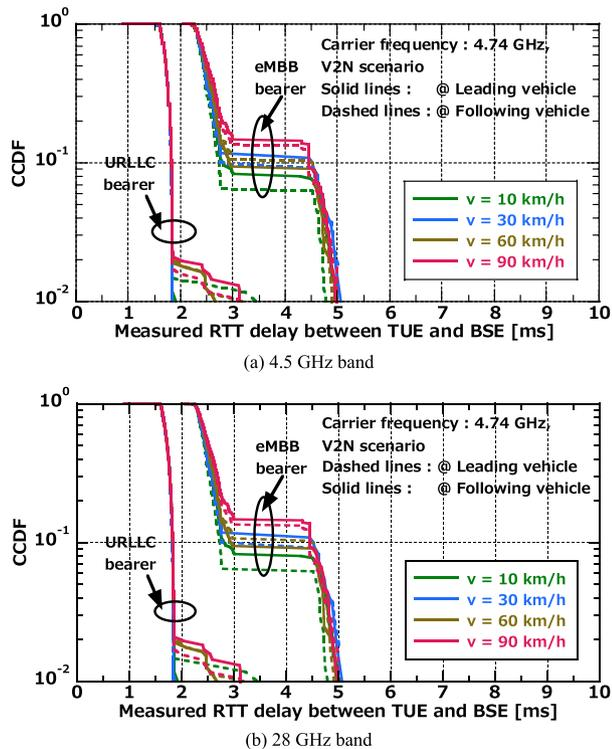
Fig. 14 Distribution of measured over-the-air latency.
