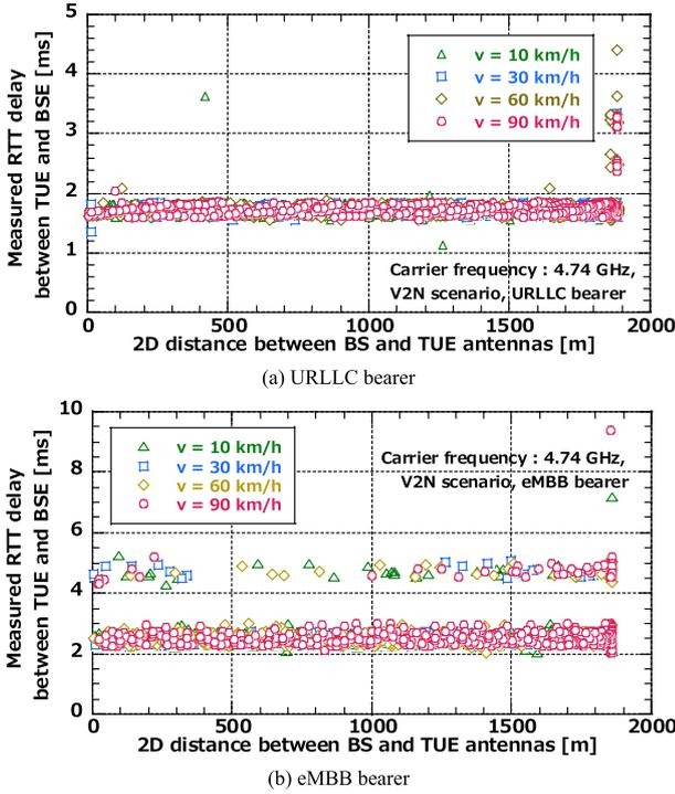
Fig. 12 Examples of latency measurement results (4.5 GHz band).
