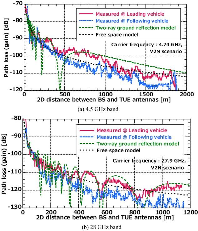
Fig. 9 Path loss evaluation results.
