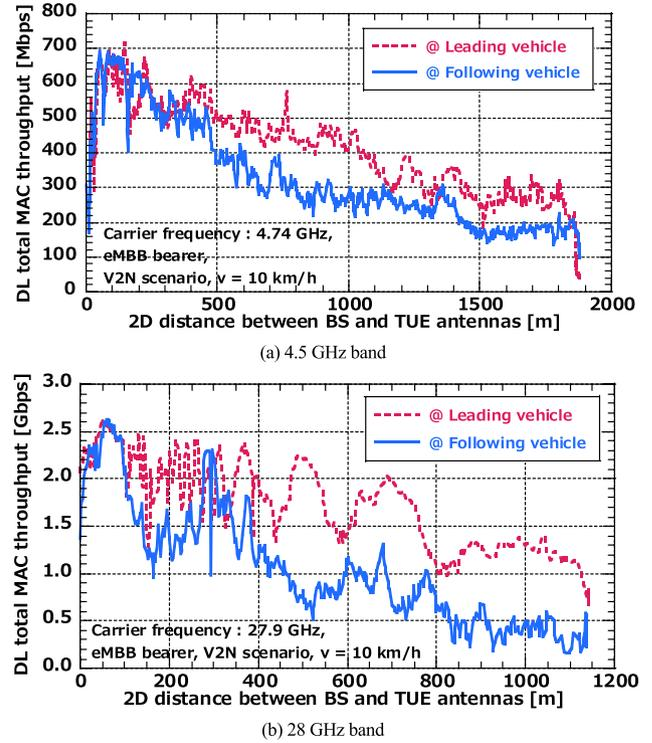
Fig. 15 Examples of over-the-air throughput measurement results.
