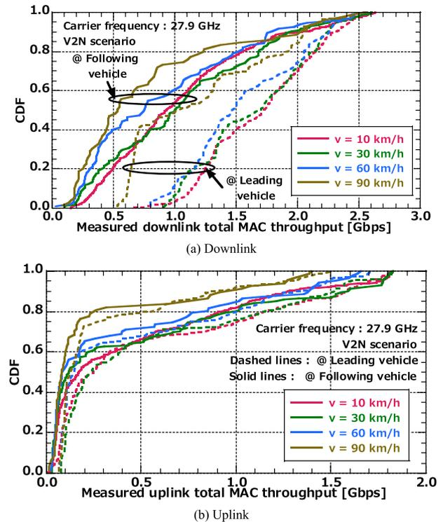
Fig. 17 Distribution of measured throughput (28 GHz band).
