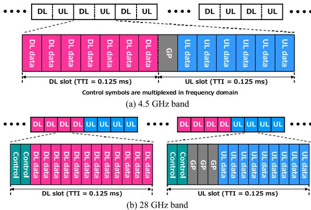
Fig. 5 Radio frame structure of prototype system.
