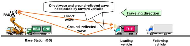
Fig. 10 Typical propagation for V2N communications at leading vehicle.
