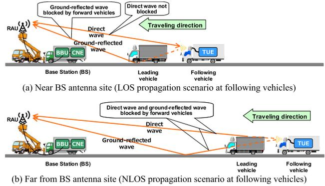
Fig. 11 Typical propagation for V2N communications at following vehicles.
