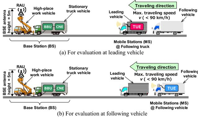
Fig. 7 Overall system setup for field evaluation.
