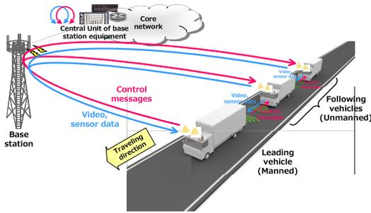
Fig. 1 Communications between vehicles in truck platooning.
