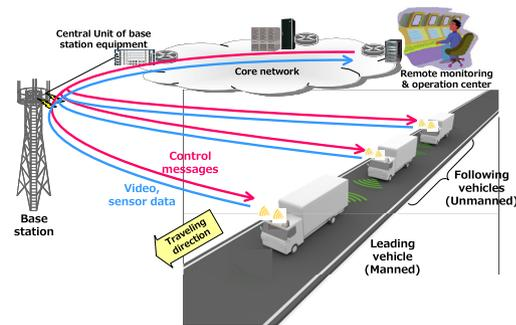
Fig. 2 Communications in remote monitoring and operations for truck platooning.
