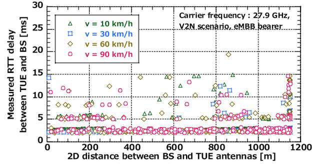
Fig. 13 Examples of latency measurement results (28 GHz band).
