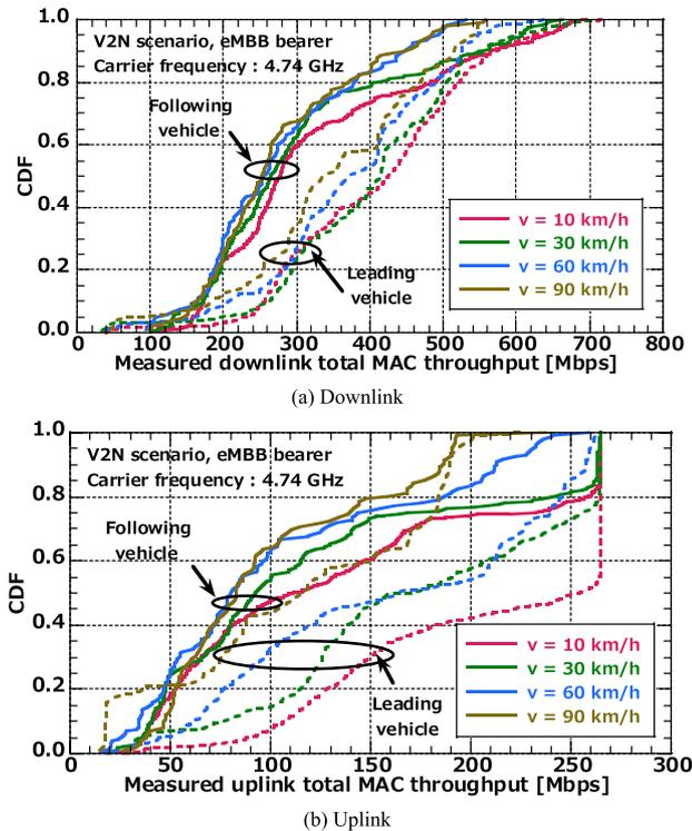
Fig. 16 Distribution of measured throughput (4.5 GHz band).
