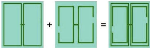
(a) Low-band antenna (b) High-band antenna (c) Dual-band antenna
