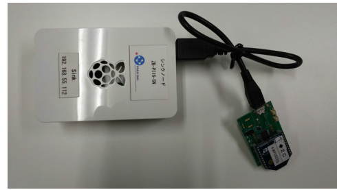
Fig. 16 Implemented sink node and cluster head node.
