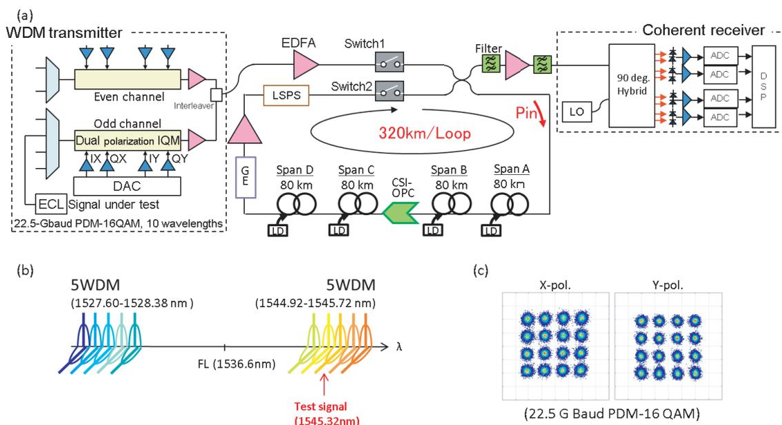
**Fig. 2** (a) Experimental setup for multi-span transmission using distributed all-Raman amplification while applying CSI-OPC to mid-span spectral inversion. (b) Arrangement of wavelength of ten WDM signals. (c) Constellation diagrams for a back-to-back signal.
