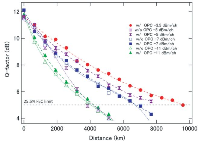
**Fig. 6** Q-factors as a function of transmission distance without and with CSI-OPC for launched powers of  $-11$ ,  $-7$ ,  $-5$ , and  $-3.5$  dBm/ch, respectively.
