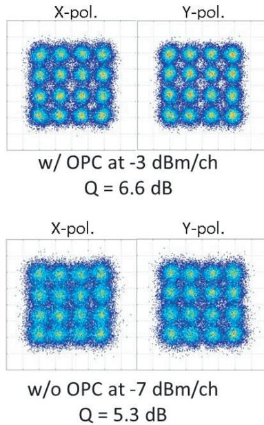
**Fig. 5** Constellation diagrams for signal with and without CSI-OPC device after 6,400 km transmission for launched powers of  $-3$  and  $-7$  dBm/ch, respectively.
