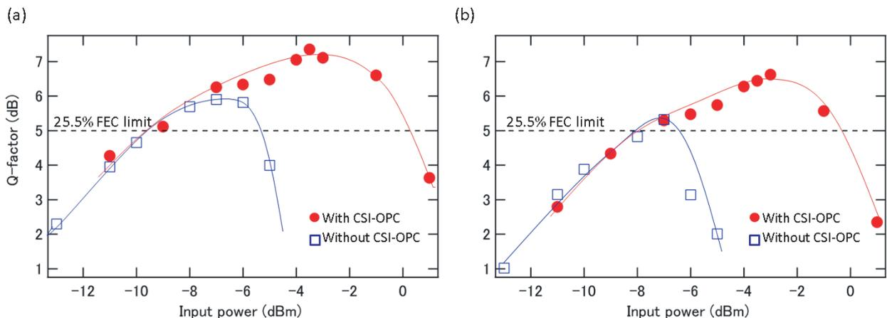
**Fig. 4** Comparison of tolerance to nonlinear impairments with and without CSI-OPC device for test signal in ten WDMs after (a) 5,120 km and (b) 6,400 km transmission.
