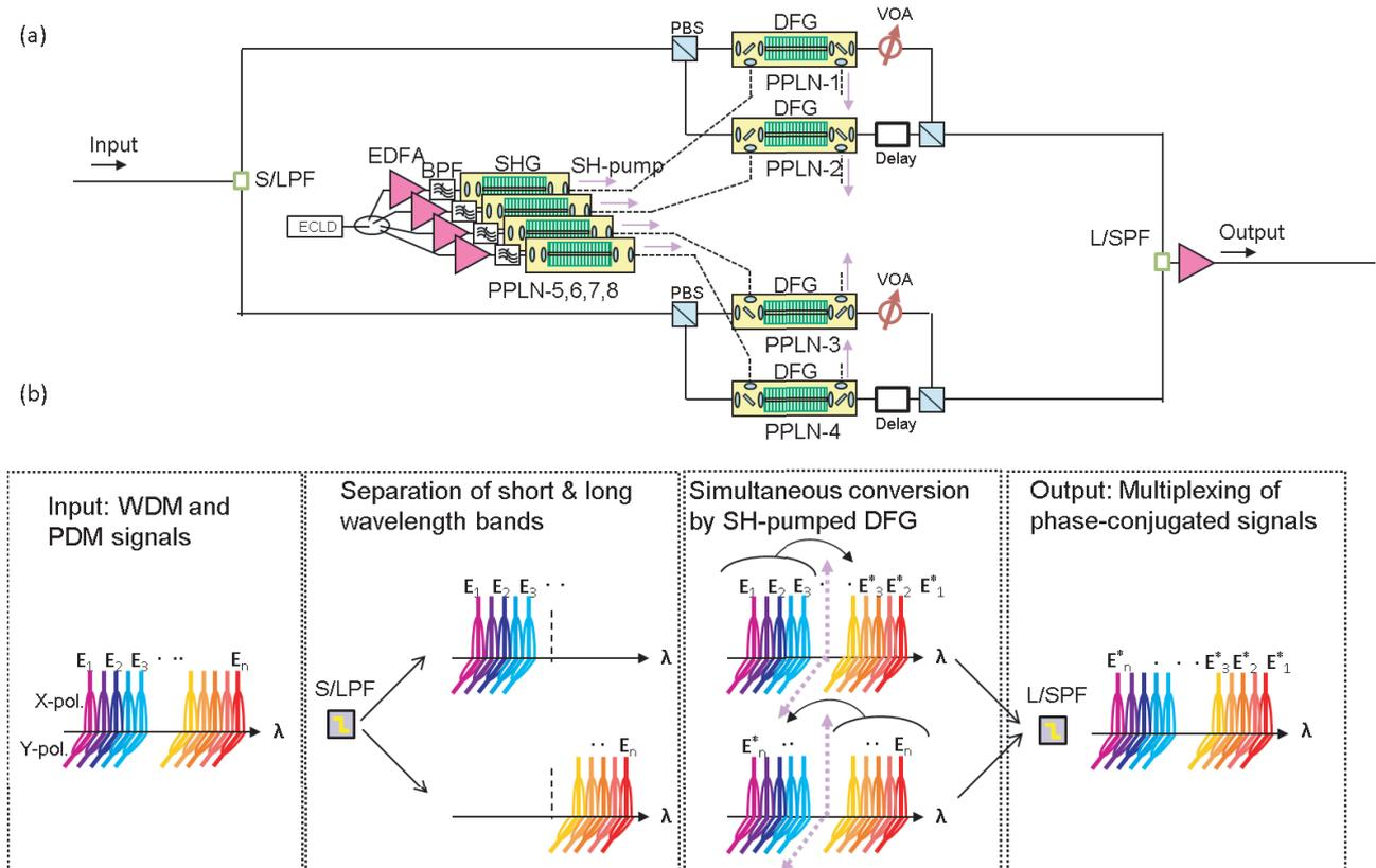
**Fig. 1** (a) Configuration of polarization-diversity CSI-OPC device. (b) Schematic diagrams of complementary spectral inversion using SH-pumped DFG.
