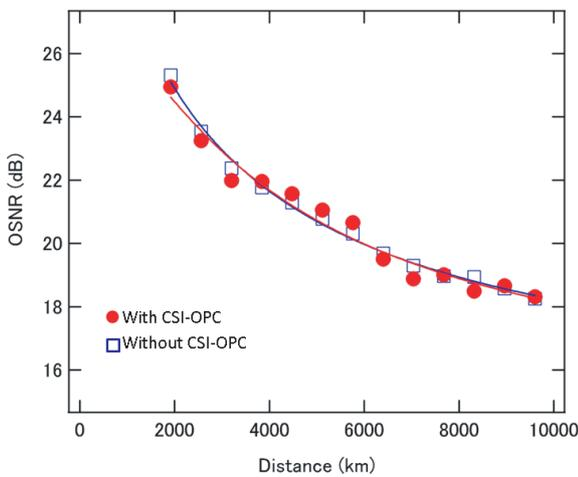
**Fig. 3** OSNRs for the recirculating loop without and with the CSI-OPC device by using CW signals with launched power of  $-7$  dBm/ch.
