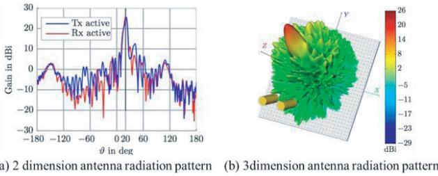
Fig. 8 Antenna radiation pattern [34].
