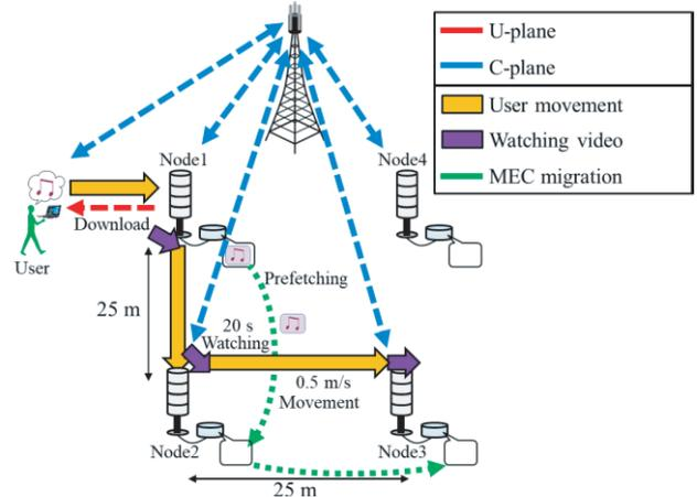
Fig. 13 Experimental environment of prefetching.
