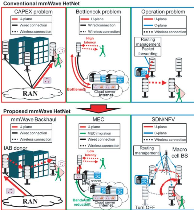
Fig. 1 Proposed approaches for SDN-based mmWave networks.
