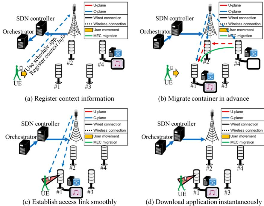
Fig. 5 Flow diagram of prefetching algorithm.
