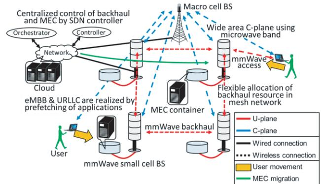
Fig. 2 SDN/NFV-based mmWave edge cloud.
