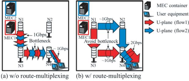
Fig. 12 Experimental environment of backhauling.
