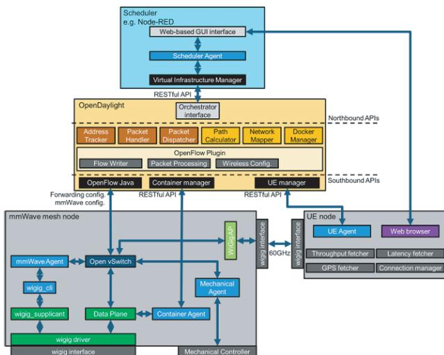
Fig. 10 Architecture of developed SDN controller.
