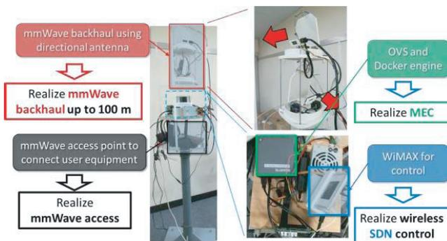
Fig. 7 Overview of hardware architecture.
