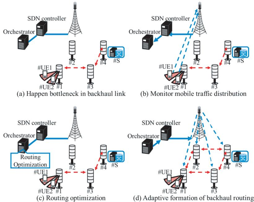
Fig. 3 Flow diagram of route-multiplexing.
