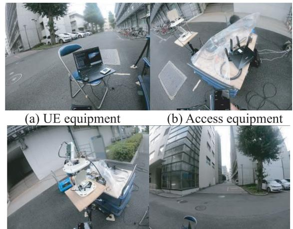
Fig. 11 Experimental environment of backhauling.
