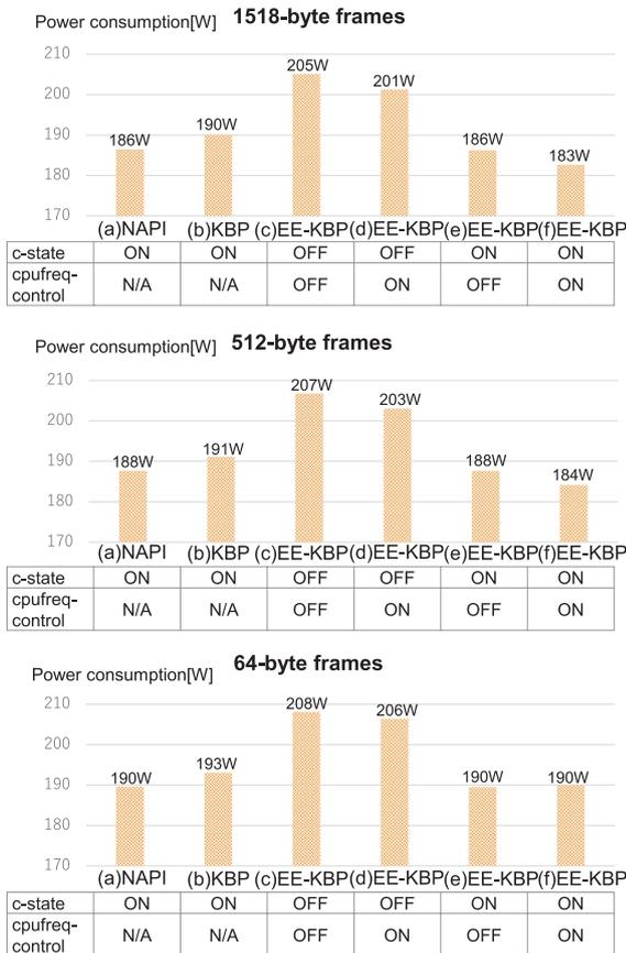
Fig. 10 Results of power consumption measurement with 1 Gbps traffic.
