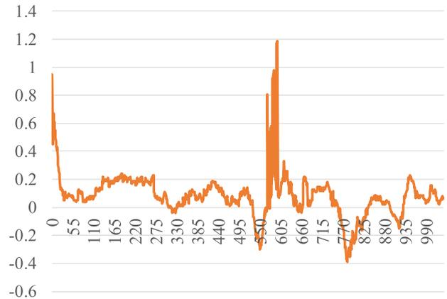
**Fig. 22** Lateral error result by road detection with recorded video on the paved road.
