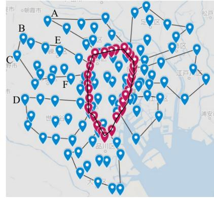
**Fig. 8** One main ring network and seven subring networks in the Tokyo metropolitan area.
