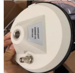
(c) Omnidirectional receiving antenna.
