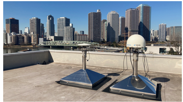
Fig. 19 Two types of GNSS antennas.
