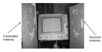
Fig. 4 Transmitter and receiver setup.
