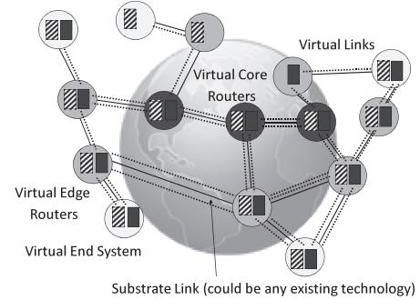
**Fig. 3** Planetary scale network virtualization (End systems (white circles), edge routers (light gray circles) and core routers (dark gray circles) are all virtualized so computational resources are isolated into different slices (solid and striped boxes). Substrate links are virtualized so network resources are also isolated.).
