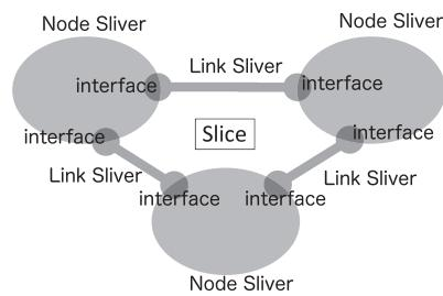
**Fig. 1** Network abstraction model in network virtualization.
