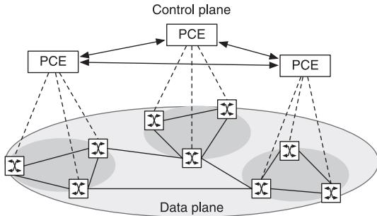
Fig. 1 Centralized wide area Ethernet.
