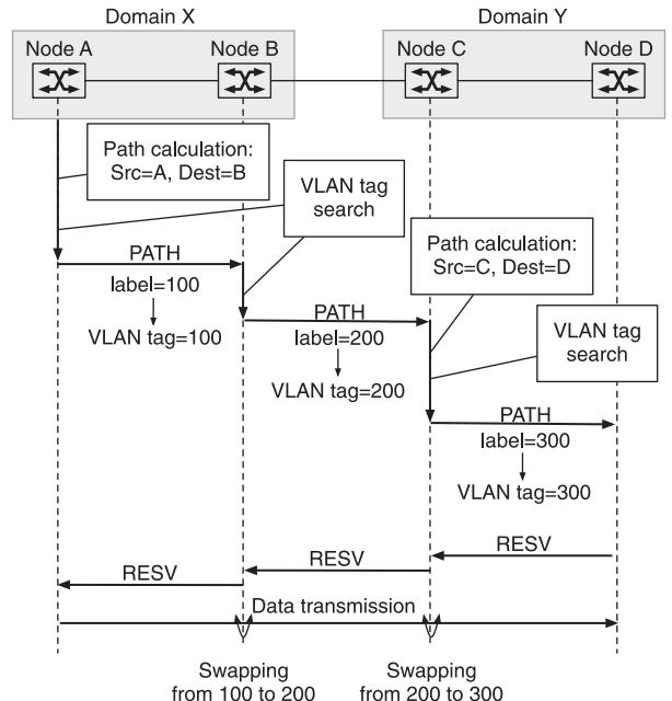
Fig. 4 Signaling sequence of L2-LSP establishment.
