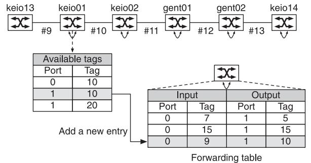
Fig. 7 Changing configurations of a switch when signaling is occurred.
