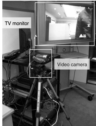
**Fig. 10** High definition video captured by video camera is displayed on TV monitor.
