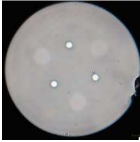
Fig. 1 Cross section of fabricated MC-EDF with 3 cores.
