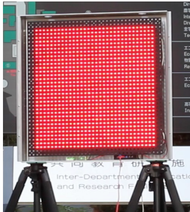
Fig. 7 1024 LED array. Each LED is arranged in a square matrix of 32 \times 32 . The size of the LED array is 465 \text{ mm} \times 465 \text{ mm} , with the LED spacing of 15 \text{ mm} . The LEDs are the same as the actual LED traffic lights in Japan.
