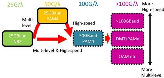
Fig. 2 Schemes for increasing transmission speed.
