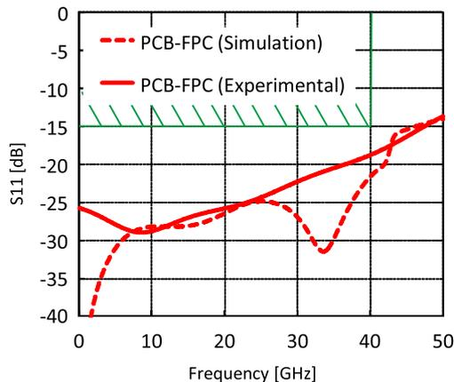
**Fig. 16** Simulation and experimental results of the reflection characteristics of the PCB to FPC connection.
