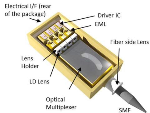
Fig. 5 Perspective view of optical multiplexer integrated with 100GbE TOSAs.
