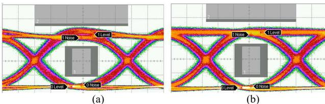
**Fig. 17** Eye pattern of EML TOSA using NRZ  $2^{31} - 1$  PRBS electrical signal at 43Gbps (a) FPC and (b) coaxial connection.
