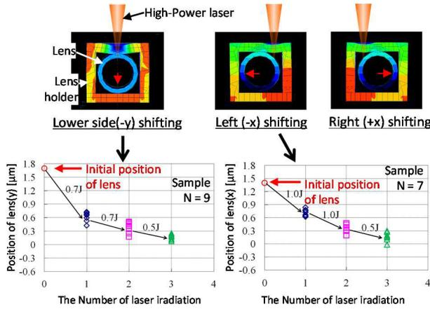
Fig. 7 Simulation and experimental results of relative position of lens as a function of the number of laser hammering.
