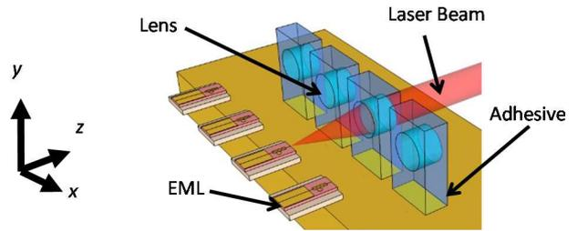
Fig. 10 Schematic diagram of optics with adhesive bonding.
