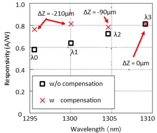
**Fig. 14** Experimental results for responsivity of the APD as a function of the wavelength with and without compensation.
