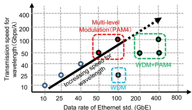
**Fig. 1** Correspondence between data rate and transmission speed per wavelength for Ethernet standards.
