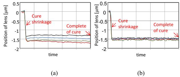
Fig. 11 Experimental results for relative position of the lens in the y-axis as a function of the duration of UV irradiation (a) before and (b) after optimizing cure conditions.
