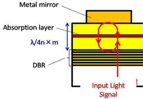
**Fig. 12** Schematic diagram of structure of resonant cavity avalanche photo diode.
