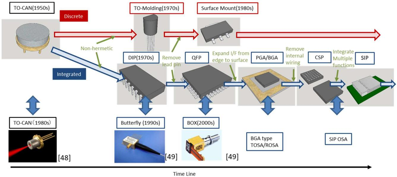
Fig. 18 Progression of package types for electrical and optical devices.
