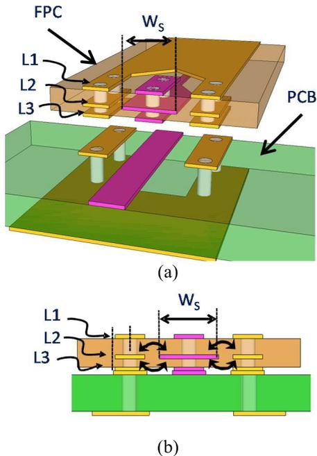
**Fig. 15** Schematic of PCB to FPC connection (a) perspective view and (b) cross-section.
