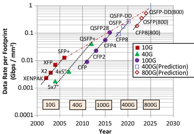
Fig. 4 Trend of transmission speed vs. footprint and time of appearance in the market.
