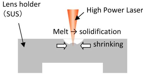
Fig. 6 Principle of laser hammering for precise lens-assembly.
