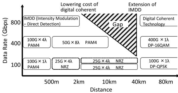
Fig. 3 Correspondence between transmission distance and data rate.
