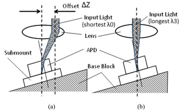
**Fig. 13** Schematic diagram of wavelength dependency compensation for an APD with a DBR structure for (a) shortest wavelength  $\lambda_0$  and (b) longest wavelength  $\lambda_3$ .
