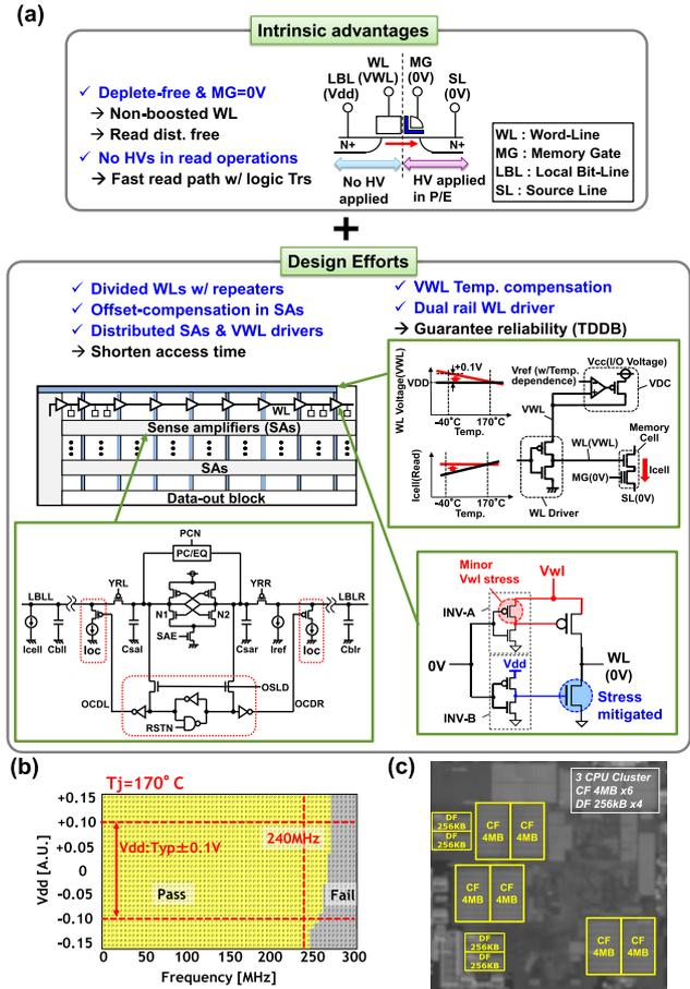
Fig. 7 SG-MONOS read path design [9]–[11]: (a) design efforts in combination with intrinsic advantages of SG-MONOS memory cells, (b) read shmoo plots of 28nm SG-MONOS code flash macro and (c) die photo of 28nm Flash MCU with SG-MONOS flash macros.
