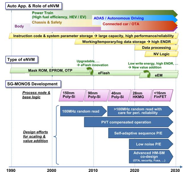
Fig. 6 Scaling scenario by device/circuit (SG-MONOS)
