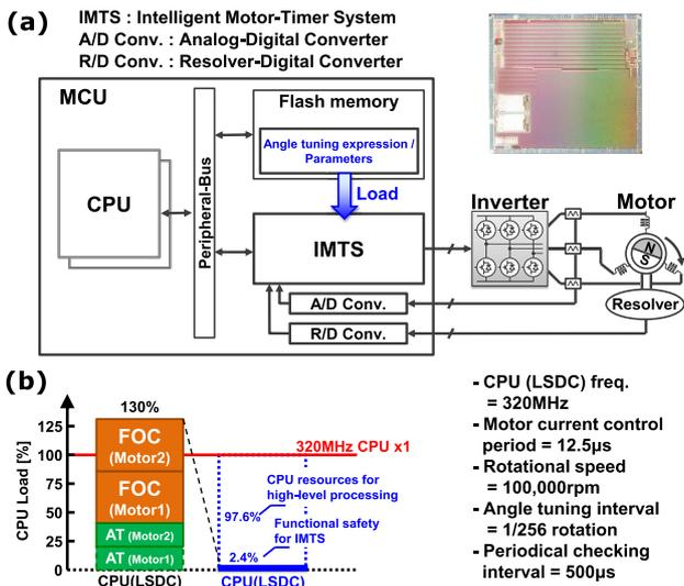
Fig. 4 Embedded flash memory use case in EV motor control [3]: (a) MCU architecture with accelerator (IMTS), and (b) Accelerator off-loads CPU very effectively by 97.6%
