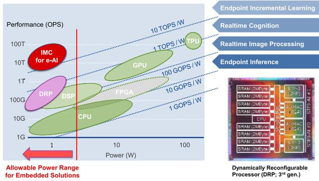
Fig. 12 Performance of processing units and AI-accelerators
