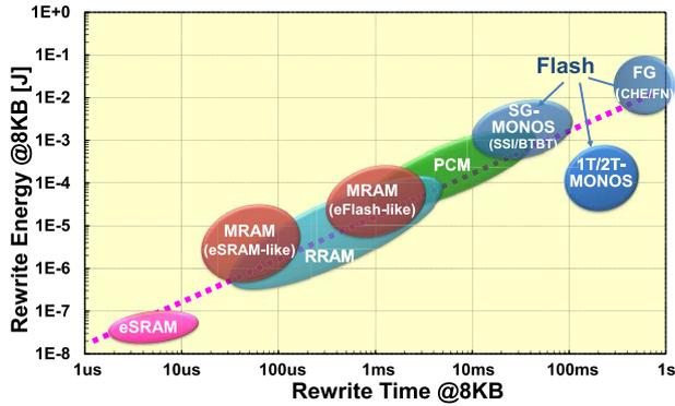
Fig. 16 Rewrite time and energy; eFlash vs eEM candidates
