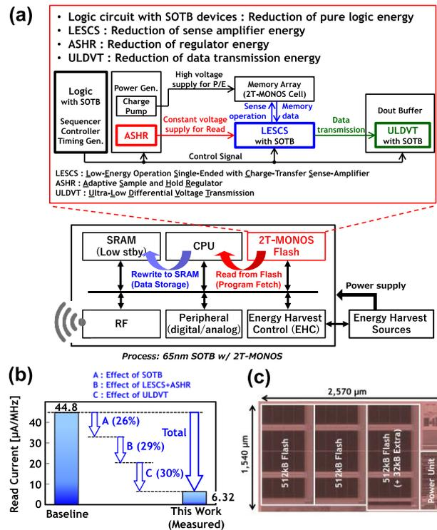
**Fig. 15** Design and achievements of 2T-MONOS eFlash macro [29]: (a) configuration of SOTB-based MCU chip and 2T-MONOS flash macro, (b) read current reduction by design efforts in 2T-MONOS flash macro and (c) photo of 2T-MONOS flash macro.
