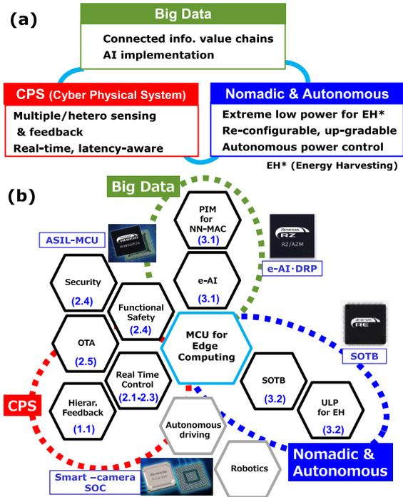
**Fig. 2** (a) Three elements of IoT, and (b) technical factors of MCU in edge computing and corresponding sub-section numbers in this paper
