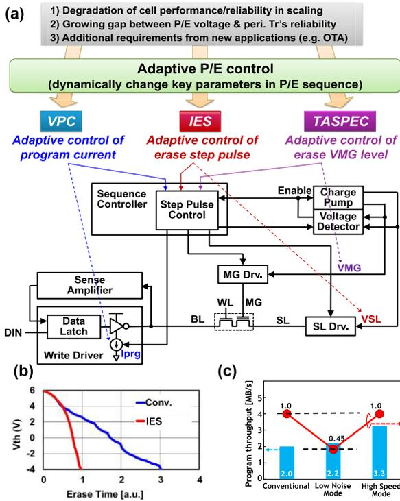
Fig. 8 Design efforts for SG-MONOS P/E operations [9]–[11]: (a) design implementation of adaptive P/E control schemes, (b) adaptive reduction of erase time by IES and (c) peak current reduction by VPC.
