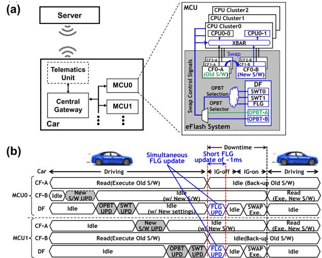
Fig. 11 RFS mechanism for OTA in automotive [10]: (a) system block diagram for OTA and (b) SW update sequence with RFS mechanism.
