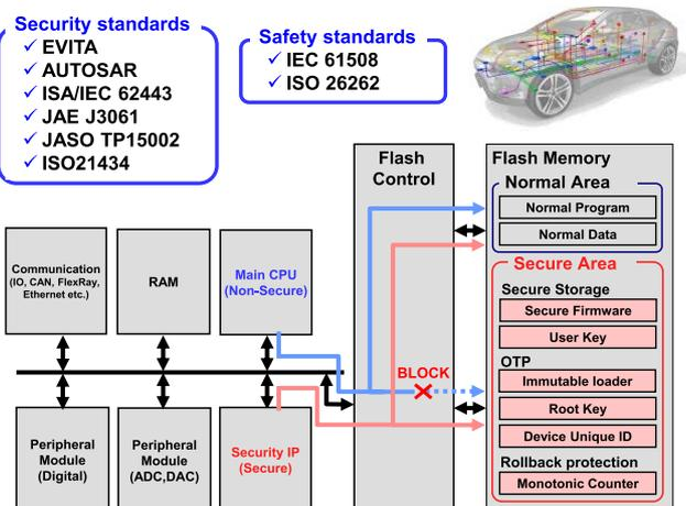
Fig. 5 Embedded flash memory use case in automotive security
