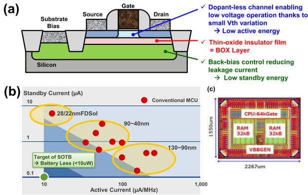
**Fig. 14** Advantages and target performance of SOTB: (a) cross-sectional view, (b) comparison of active/standby current with conventional technologies and (c) SOTB MCU test chip [27].
