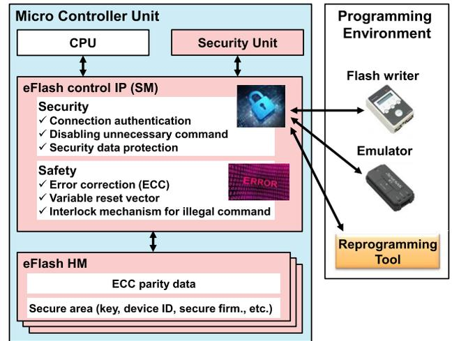
Fig. 9 Security and safety functions for eFlash sub-system
