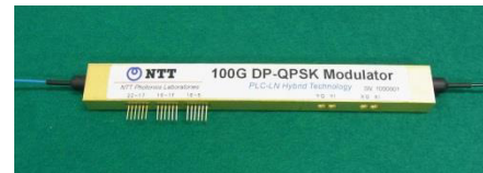
Fig. 4 Photograph of silica-LN DP-QPSK modulator which size is 118 mm long, 13.5 mm wide, and 7 mm height.
