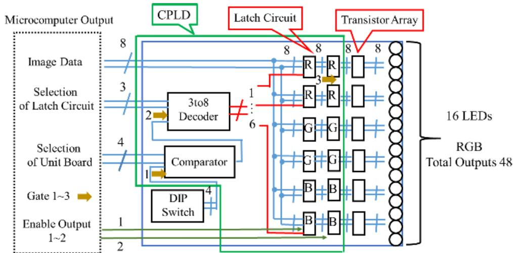
Fig. 3 Configuration diagram of the sub board.
