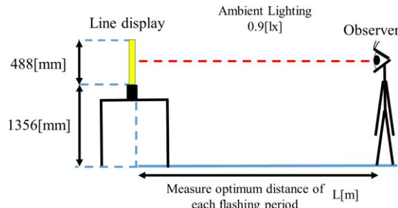
Fig. 10 Experimental condition for optimal distance.
