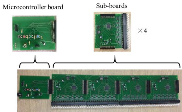
Fig. 6 Connected the microcontroller board to the sub board.
