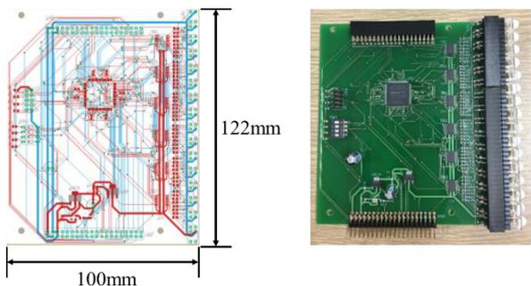
Fig. 5 Pattern diagram designed by CDA software Eagle and the developed sub-board.
