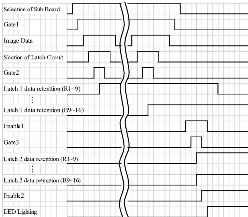
Fig. 4 Timing diagram of data transfer for LEDs.
