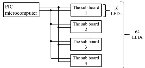
Fig. 2 Configuration diagram of line display.
