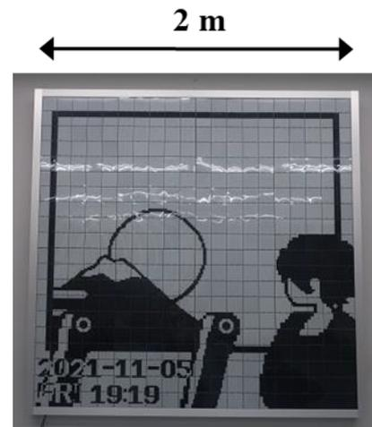
**Fig. 7** Prototype of 2 m × 2 m square panel formed with 400 e-Tiles.
