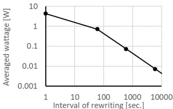
**Fig. 12** Averaged wattage of 4 m<sup>2</sup> display area using e-Tile when all-OFF state is inserted between rewriting timing longer than 60 sec.
