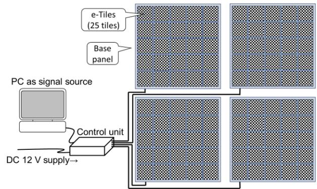
**Fig. 6** Basic construction of the prototype display system using e-Tile.
