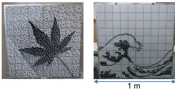
**Fig. 5** Prototype of 1 m square panel [constructed with 100 e-Tiles].
