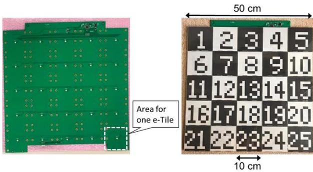
**Fig. 4** Base panel for arraying 25 e-Tiles.
