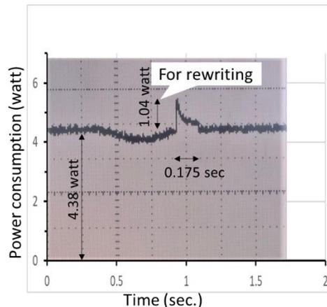
**Fig. 11** Power consumption indicated by a driving wave form for 4 m<sup>2</sup> display area using e-Tile.
