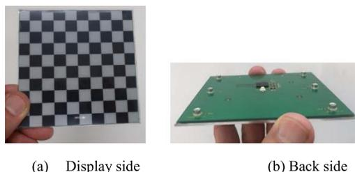
Fig. 3 Prototype of e-Tile.
