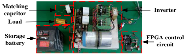
Fig. 9 The physical picture of the transmitter circuit.
