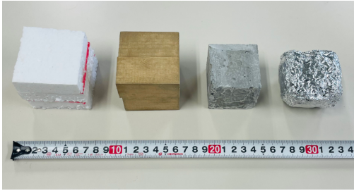
(c) four types of buried objects (from left to right: styrene foam, wood, concrete, and aluminum)
