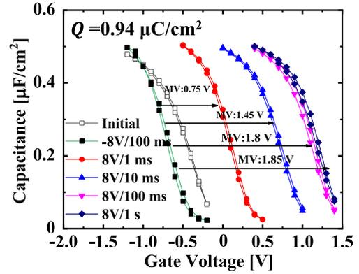
**Fig. 7** The charge trap operation utilizing program pulse of  $V_{PGM}/t_{PGM} = 8$  V/1 ms–1 s. The C-V characteristics were measured at 100 kHz. The schematic measurement sequence was also shown.
