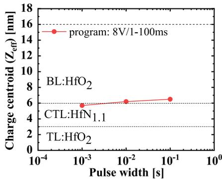
**Fig. 6** Pulse width dependence on  $Z_{eff}$ .
