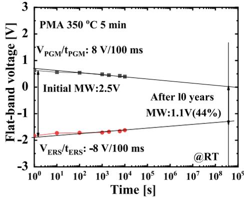
**Fig. 5** Retention characteristic for charge trap operation of FeNOS diode with PMA at 350°C/5 min. The input pulses were  $\pm 8$  V/100 ms for charge trap operation.
