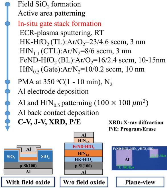
Fig.2 Fabrication process for Al/HfO<sub>0.5</sub>/HfO<sub>2</sub>/HfN<sub>1.1</sub>/HfO<sub>2</sub>/Si(100) FeNOS diodes. Schematic cross-sections and plane-view were also shown.
