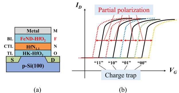
**Fig. 1** (a) Schematic cross-section of the FeNOS NVM and (b) schematics of  $V_{TH}$  control in FeNOS NVM. The partial polarization of FeND-HfO<sub>2</sub> BL realizes the analog control of  $V_{TH}$  (dotted lines) along with the multi-bit/cell operation of the charge trap in the HfN<sub>1.1</sub> CTL (solid lines).
