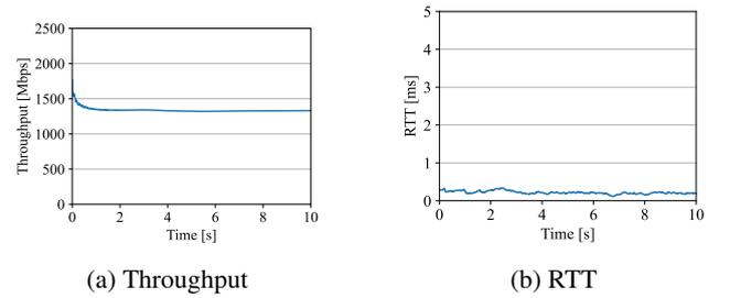
Fig. 5: Network performance with lossless compression (H.265) via wired connection
