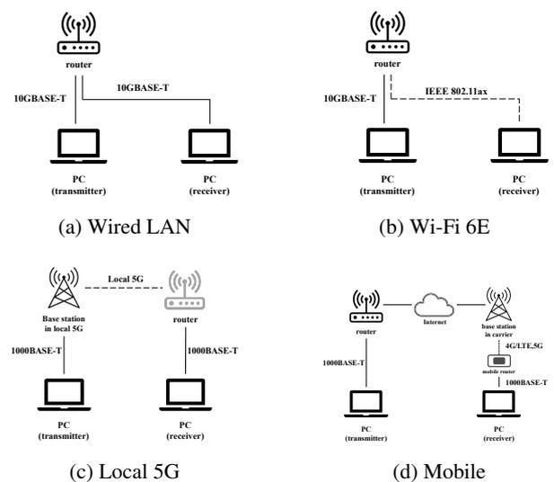
Fig. 3: Network connections in each network
