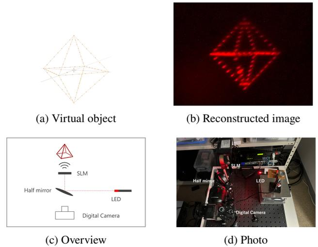
Fig. 2: Optical system for reconstruction
