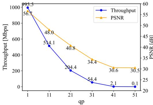
Fig. 6: Throughput and PSNR with lossy compression (H.265)
