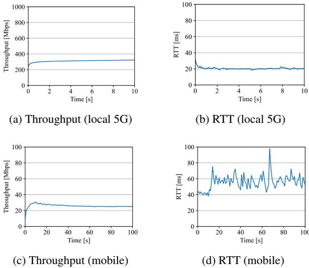
Fig. 9: Network performance with no compression via local 5G and mobile networks
