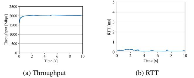
Fig. 4: Network performance with no compression via wired connection
