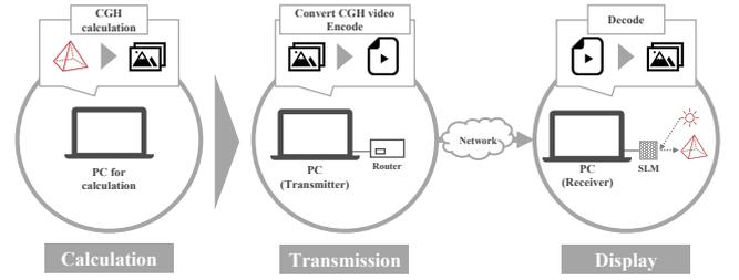
Fig. 1: Overview of developed streaming system for CGH video
