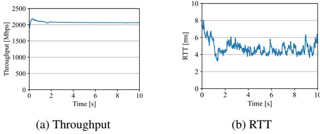
Fig. 8: Network performance with no compression via Wi-Fi 6E
