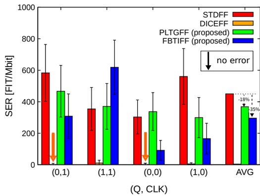
Fig. 23: n-SER under four (Q, CLK) states and average. Error bars are within 95% confidence.
