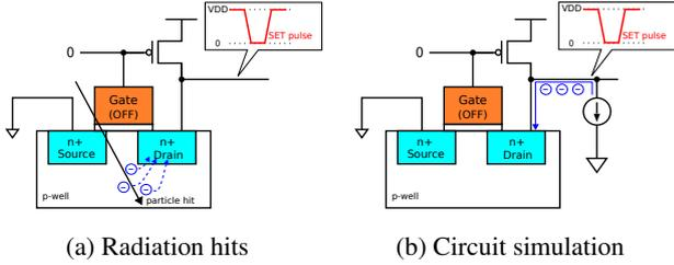
Fig. 5: Charge collection is emulated by a current source in circuit simulation.
