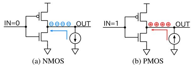
Fig. 4: Schematic to obtain  $Q_{crit}$  of each transistors.
