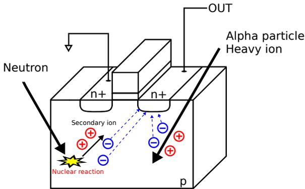
Fig. 1: Single event effect on a silicon devices.
