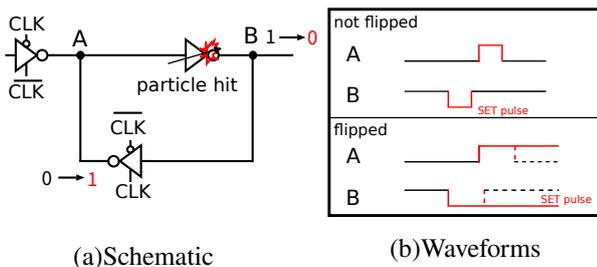
Fig. 2: Soft error mechanism in a latch.
