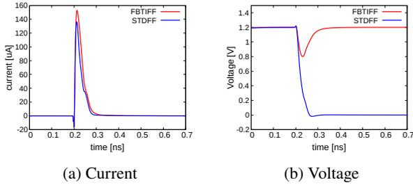
Fig. 16: The current and voltage waveforms at node ① when heavy ions ( LET = 1.4 MeV·cm<sup>2</sup>/mg ) are irradiated at the midpoint between T1 and T2.
