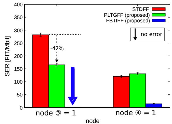
Fig. 22:  $\alpha$ -SER results considering the difference in  $(Q, CLK)$  between STDFF and the proposed circuits. To facilitate comparison of the results of the STDFF and the proposed circuit, it shows the error rate for each node when the value of each node is 1.
