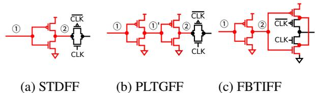
Fig. 11: The signal path from node ① to the pass transistor that connects PL and SL.
