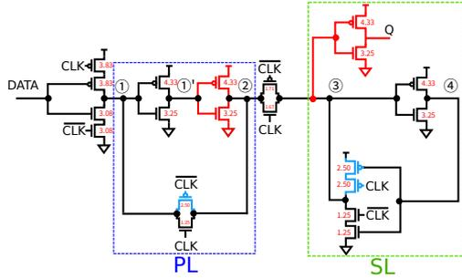
Fig. 7: Primary Latch Transmission Gate FF (PLTGFF)
