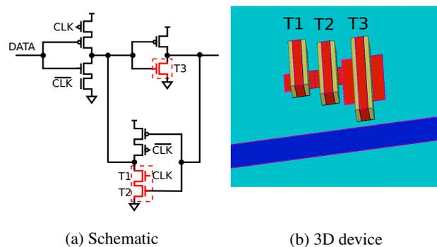
Fig. 12: Schematic and 3D device structure on TCAD.
