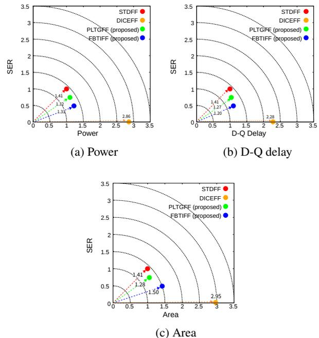
Fig. 26: 2 dimensional charts of soft error tolerance and each performance (Area, D-Q delay, Power). SER is the sum of  $\alpha$ -SER and n-SER. SER and each performance are normalized by the STDFFF value.
