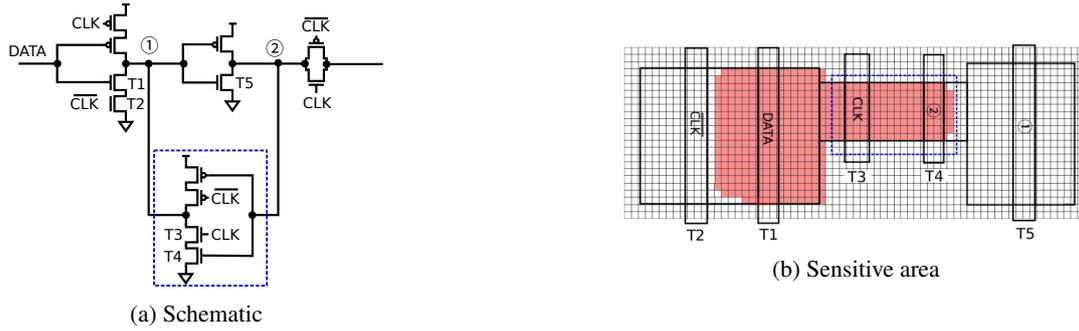
Fig. 13: Shape of sensitive area in PL of STDFF by heavy ions with LET of  $1.4 \text{ MeV}\cdot\text{cm}^2/\text{mg}$ .
