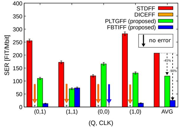
Fig. 21:  $\alpha$ -SER under four  $(Q, CLK)$  states and average  $\alpha$ -SER. Error bars are within 95% confidence. These results assume the use of the super ultra low alpha (SULA) package ( $0.001$  cph/cm<sup>2</sup>). Note that DICEFF has no error at all conditions.
