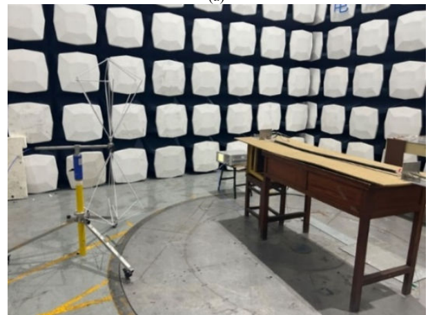
Fig. 4 (a) Arrangement of the scaled short-line model measurement for PLC, and (b) measurement in the anechoic chamber.
