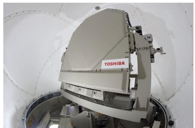
Fig. 1 Photograph of the Dual Polarization Phased Array Weather Radar in Osaka University. At the top of the building in the electrical engineering department, the radar facilities of planar array configuration are equipped.
