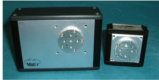
Fig. 16 Photograph of ASK transceiver (left) and receiver (right) for distribution of uncompressed high-definition TV signal with data rate of 1.5 Gbps.
