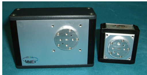
Fig. 16 Photograph of ASK transceiver (left) and receiver (right) for distribution of uncompressed high-definition TV signal with data rate of 1.5 Gbps.
