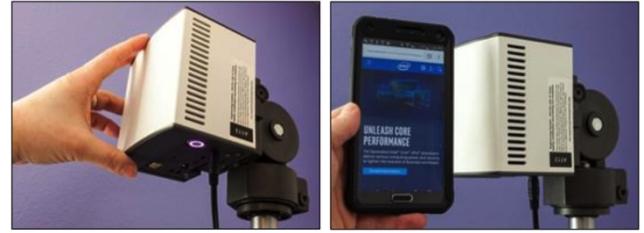
Fig. 18 Prototype hardware for mmWave mesh node.
