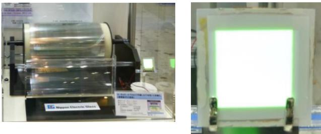
**Fig. 10** Device structure and an emitting picture of the developed flexible OLED device. The roll type ultra-thin glass with ITO fabricated by the process shown in Fig. 3 is also shown.
