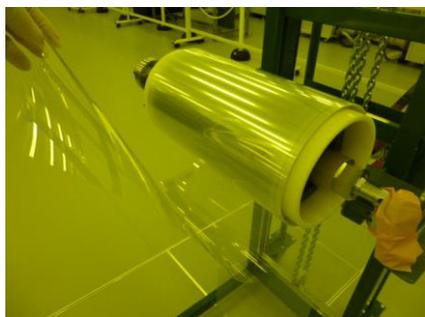
Fig. 1 Roll-type flexible ultra-thin glass OA10G supplied from Nippon Electric Glass.
