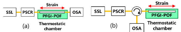
Fig. 8 Actual experimental setups of (a) transmissive configuration and (b) reflectometric configuration. OSA, optical spectrum analyzer; PFGI-POF, perfluorinated graded-index polymer optical fiber; PSCR, polarization scrambler; SSL, swept-source laser. The yellow lines indicate silica single-mode fibers.
