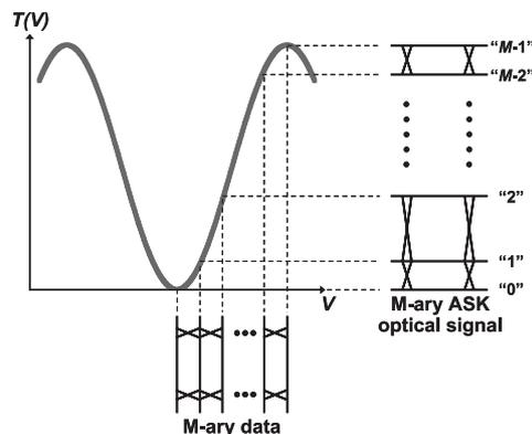
Fig. 3 M-ary ASK using LN intensity modulator.
