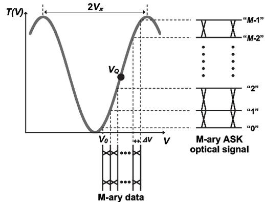
**Fig. 8** M-ary ASK model for conventional transmitter.
