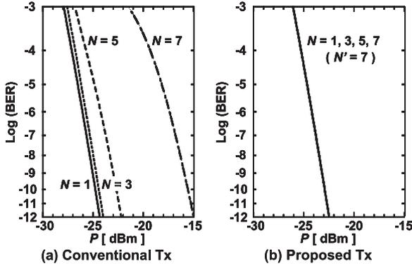
Fig. 9 BER characteristics at 1.25 Gbit/s against average optical power per wavelength,  $P$ , when  $K = 8$ .
