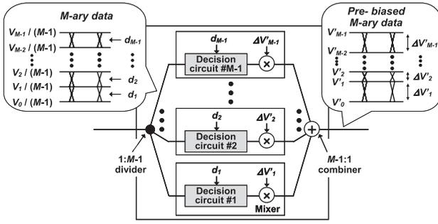
Fig. 6 Pre-biasing circuit.
