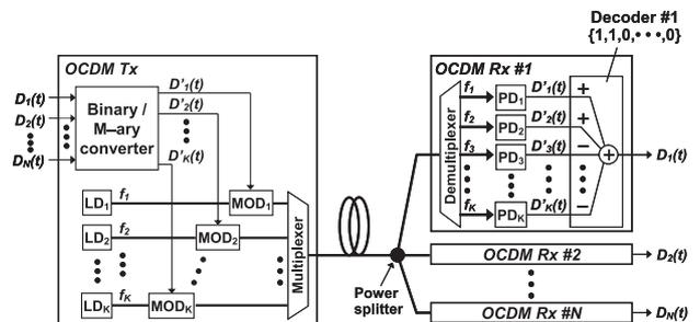
Fig. 2 Configuration for spectral M-ary ASK OCDM.
