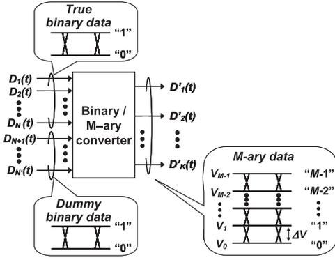
Fig. 5 M-ary data generation at binary/M-ary converter employing dummy data input.
