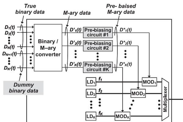
Fig. 4 Proposed transmitter configuration employing pre-biasing circuits and dummy data input.
