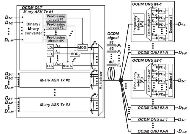
Fig. 10 Future optical access network based on spectral M-ary ASK OCDM.
