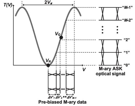
Fig. 7 M-ary ASK using LN intensity modulator with pre-biasing.
