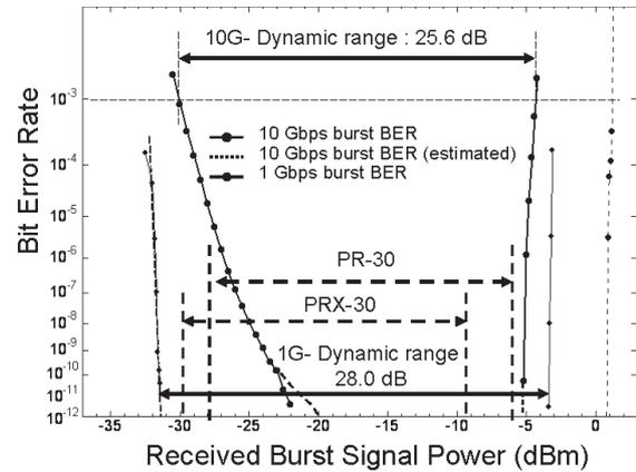
**Fig. 8** BER characteristics of the dual-rate burst mode receiver.
