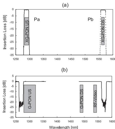
Fig. 6 Transmission characteristics of the WDM1r; (a) NG-PON ports, Solid line shows port Pa and dashed line shows port Pb, (b) G-PON port.
