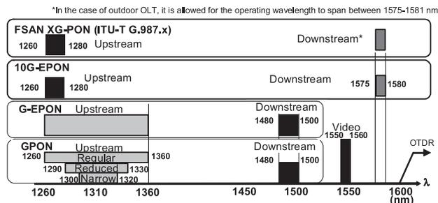
Fig. 2 Wavelength allocation of G/GE-PON and 10G-E/XG-PON.
