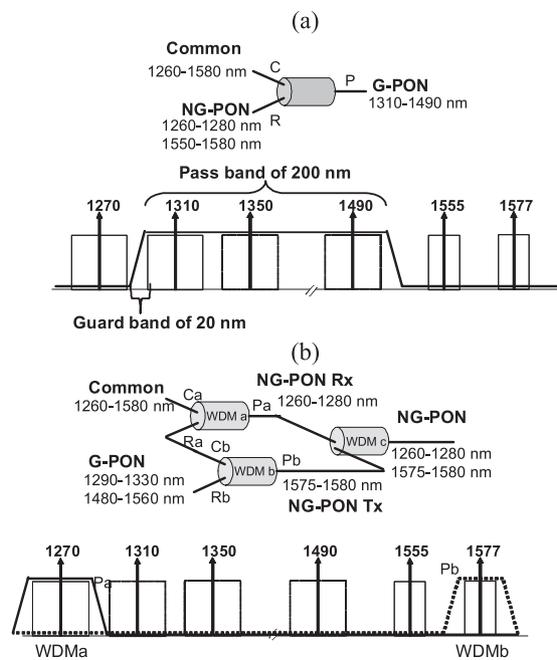
Fig. 5 Examples of WDM filter for co-existence G-PON and NG-PON: (a) Single pass band type, and (b) Combination of two kinds of band pass filter.
