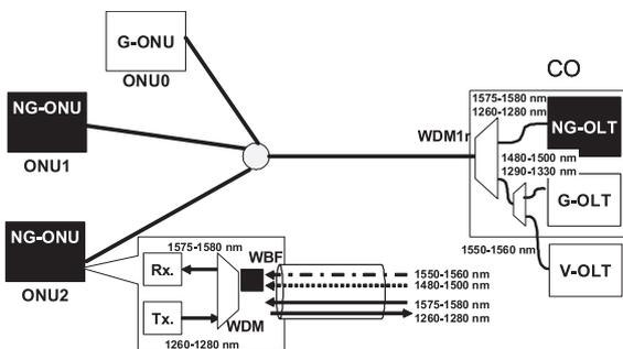
Fig. 4 Co-existence of deployed system with NG-PON via WDM.
