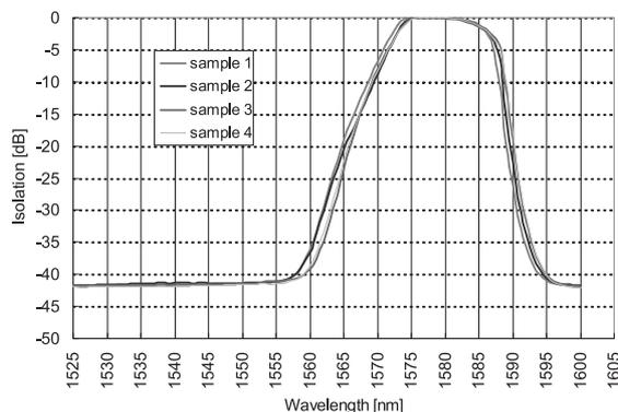
Fig. 7 Isolation characteristics of the WBF for ONU.
