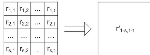
Fig. 4 Condensation of  $s \cdot t$  pixels to one concentrated pixel.
