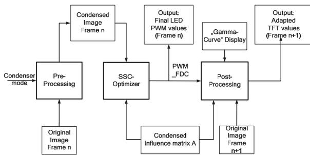
Fig. 7 Diagram of pre-processing, SSC and post-processing.
