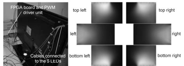
Fig. 9 Prototype (left) with measured LSFs (right).
