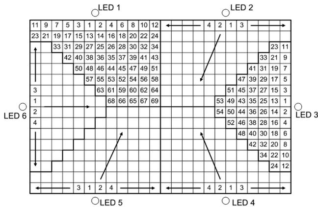
Fig. 2 Separation of an edge-lit display in six sectors.
