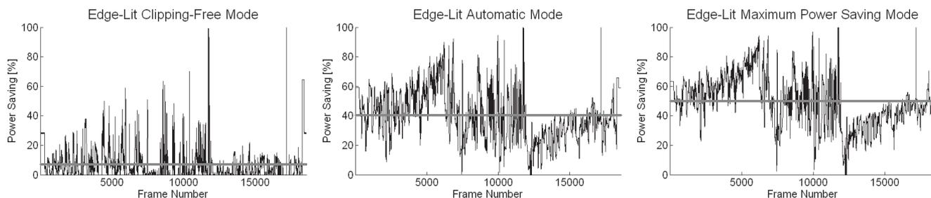
**Fig. 15** Power saving of edge-lit display (from the left): Clipping-free mode, automatic mode, maximum power saving mode).
