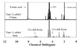
**Fig.6** Analysis of by-product by photo resist decomposition using 1H-NMR.
