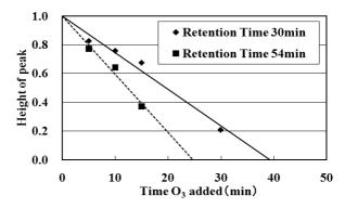
Fig. 5 Time O<sub>3</sub> added and peak height of novlak resin using HPLC.
