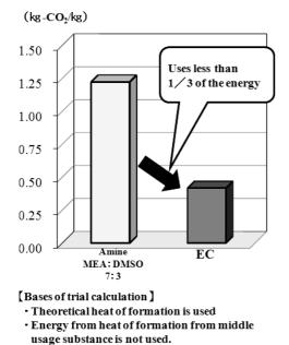
Fig. 2 Comparison of CO<sub>2</sub> emission between strippers.
