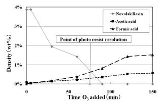
**Fig. 7** Relationship between O<sub>3</sub> adding time and by-product using 1H-NMR.
