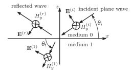
**Fig. 1** Reflection and transmission of a TM plane wave by a flat interface (z = 0) between media 0 and 1.
