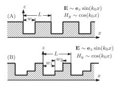
**Fig.6** Examples of perfectly conductive step gratings which support guided standing waves, when the period *L* and groove widths w,  $w_1$ ,  $w_2$  are integer multiples of  $\lambda/2$ ,  $\lambda$  being wavelength.
