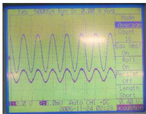
(c)The optical signal is modulated in phase with S2 element.
