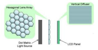
**Fig.3** Autostereoscopy with a directional backlight using a tilted convex lens array and a vertical diffuser.
