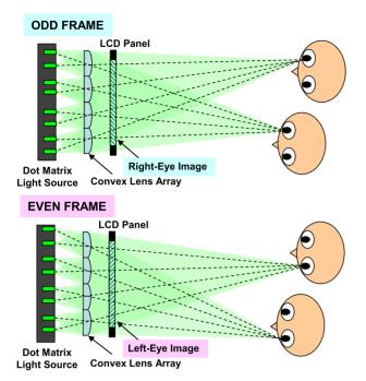
Fig. 1 Autostereoscopy with a directional backlight using a convex lens array
