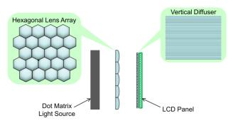
**Fig.2** Autostereoscopy with a directional backlight using a convex lens array and a vertical diffuser.
