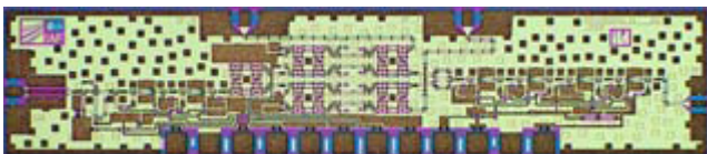
Fig. 5 Circuit architecture and chip photograph of the 300 GHz receive MMIC. Chip size is 0.75 \times 3.25 \text{ mm}^2 .
