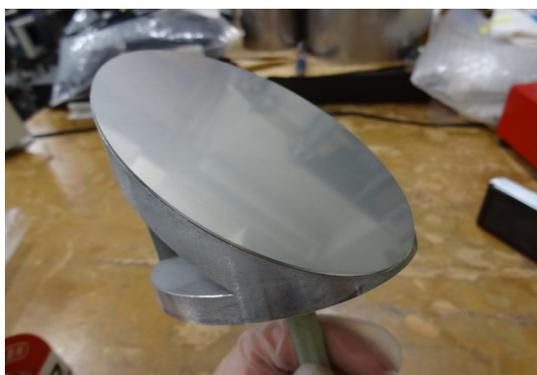
Fig. 9 Photograph of the polarization mirror made by SUS-316L.
