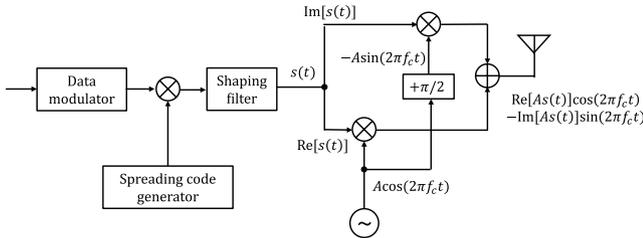
Fig. 7 System model of DS-CDMA transmitter.
