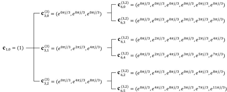
Fig. 5 Code tree for the proposed complex OVFSF (3, 2) code.
