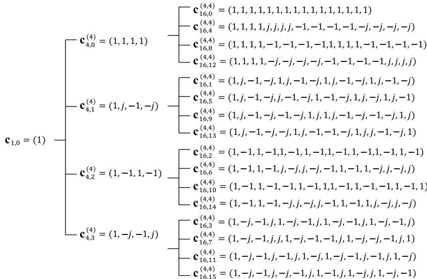
Fig. 4 Code tree for the proposed complex OVFSF (4, 4) code.
