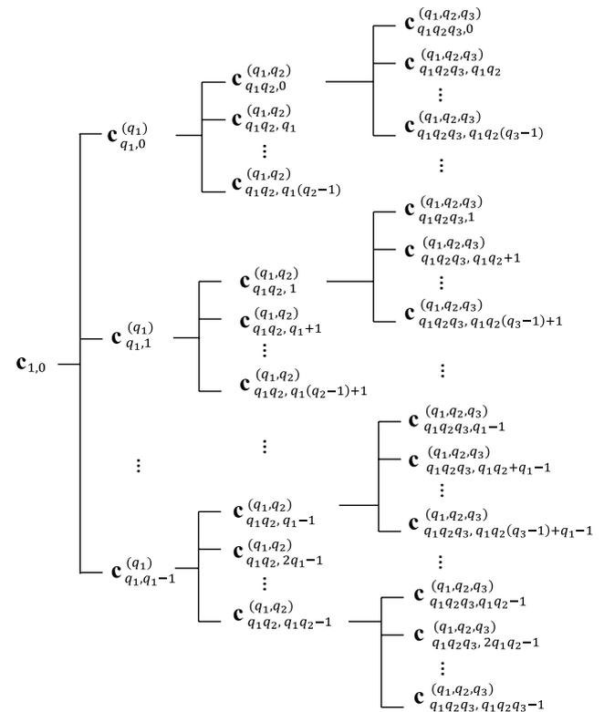
Fig. 2 Code tree for the proposed complex OVFS  $(q_1, q_2, q_3)$  code.
