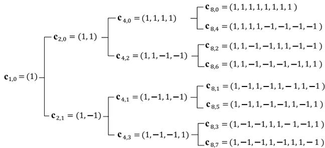
**Fig. 1** Code tree for the conventional OVSF code with  $L = 3$ . This code is also represented as the complex OVSF  $(2, 2, 2)$  code.
