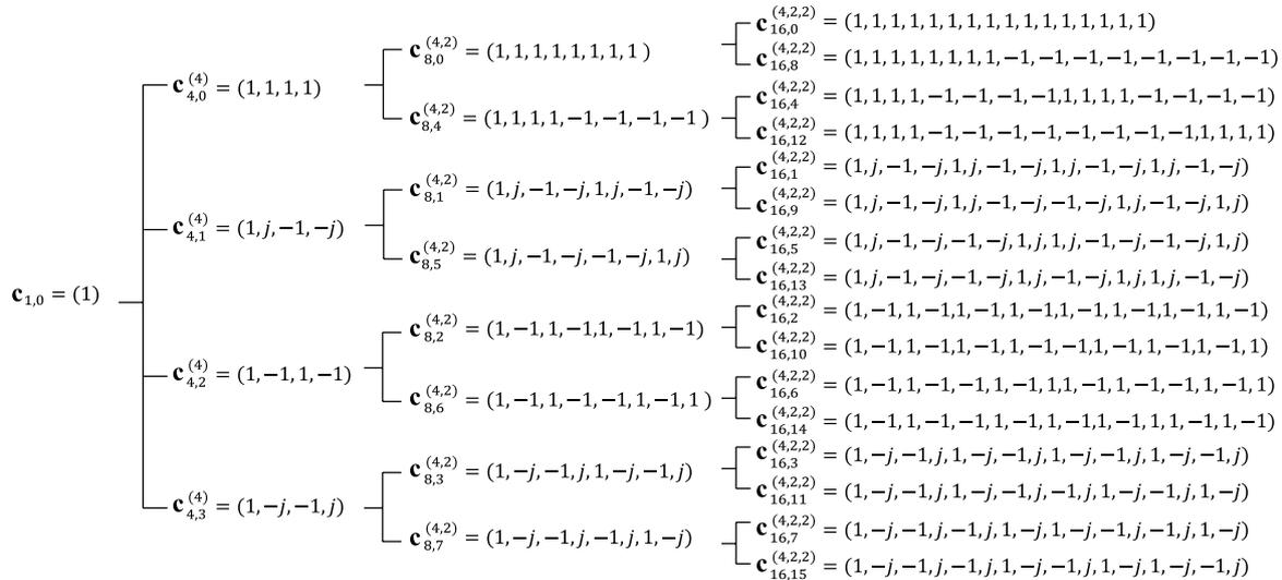
Fig. 3 Code tree for the proposed complex OVFSF (4, 2, 2) code.
