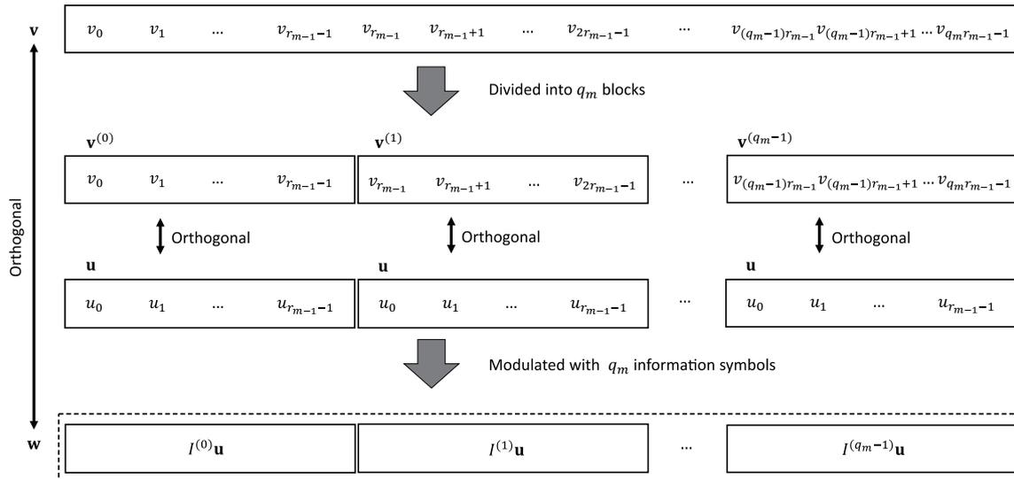
**Fig. 6** Code orthogonality. Two sequences  $\mathbf{v}^{(k)}$  and  $\mathbf{u}$  are mutually orthogonal for  $0 \leq k \leq q_m - 1$ , and two sequences  $\mathbf{v}$  and  $\mathbf{w}$  are mutually orthogonal for any information symbols  $I^{(0)}, I^{(1)}, \dots, I^{(q_m-1)}$ .
