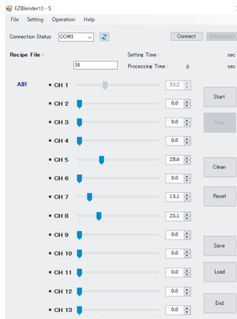
Fig. 2 GUI to specify relative concentration and delivery time of each component (EZ Blender).
